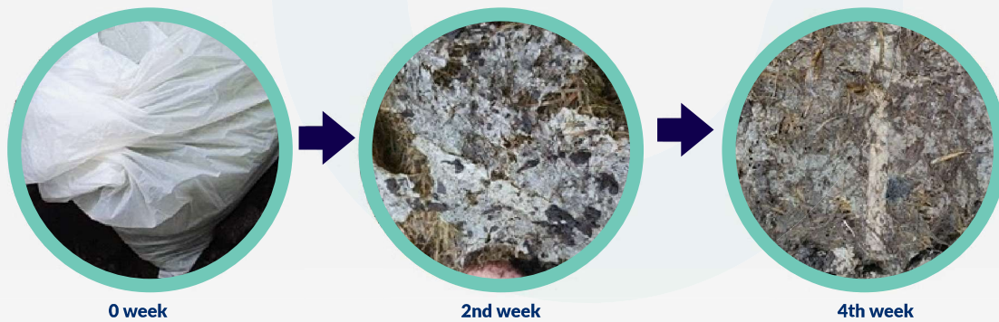
Disintegration test of ROSECO Bio-compost compound (according to ISO 16929)
